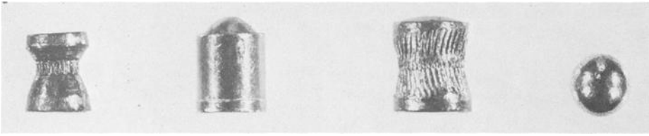
FIG. 2—A comparison of air and spring gun pellets and BB shot. Left to right: 4.5 mm (0.177 in.), 5 mm (0.20 in.), 5.5 mm (0.223 in.) and spherical BB shot (4.5 mm or 0.177 in.).
